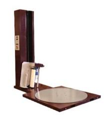
**High Profile Turntable** - The high profile machine has a raised turntable, usually 11" - 12" from the floor to the turntable, and can only be loaded with a forklift truck! There is no possibility of loading a high profile machine with a pallet jack. The high profile machine can be interfaced with a pallet conveyor line to feed pallets directly onto the wrapping machine turntable.
