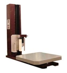
Rotary Arm Machines – The rotary arm machine is designed to wrap pallets directly on the floor. The arm rotates around the pallet, so the pallet does not move. You eliminate the need to push a load up a ramp by hand to place it in position for wrapping. This is system is very effective for loads that are either very heavy, or light and unstable, or irregularly shaped loads.
